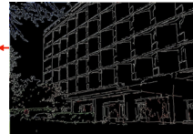
Canny Edge Detector: Edge Filter: Gaussian Filter: Sobel Operator: Non Max Suppression: Double Thresholding: Edge Tracking
