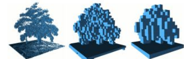
Fig. 3 By limiting the depth of a query, multiple resolutions of the same map can be obtained at any time. Occupied voxels are displayed in resolutions 0.08 m, 0.64, and 1.28 m.
