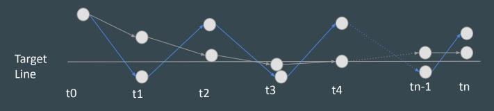
Target Line  $Distance to line \\ time \\ Controller \\ steer_t = 0.3 2 * d$   $Controller \\ towards \\ line \\ Location - x$
